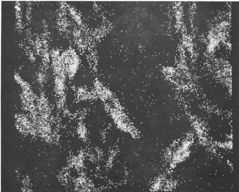
Fig. 12. Computer enhanced aluminum Auger map of the fractured surface.
